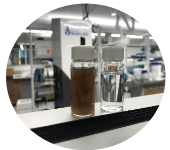
Wastewater before and after treatment
