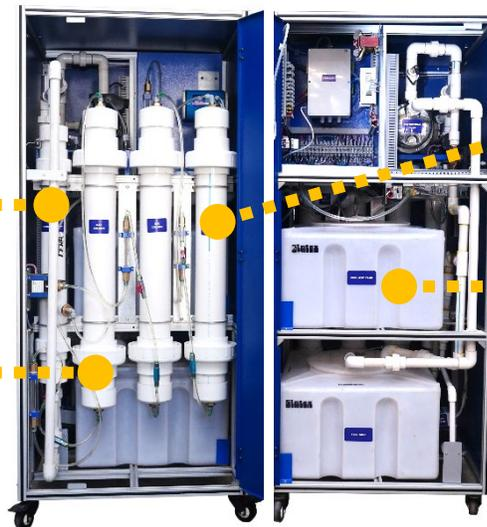
Designed to treat blackwater to ISO 30500, treated water can be re-used for multiple purposes, including flushing, irrigation and laundry.
